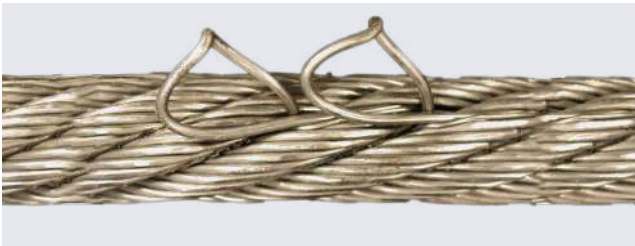
Protruded wires of inner rope
