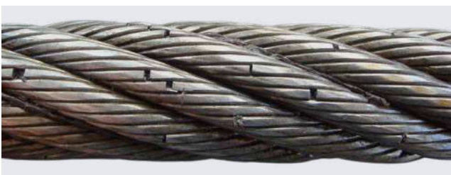
Crown wire breaks
