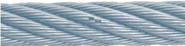
Figure 38: Condition at 40% of the bending cycle until breaking point
