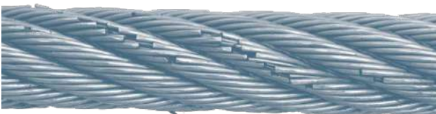
Figure 40: Condition at 80% of the bending cycle until breaking point
