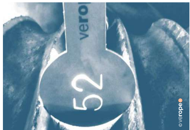
Figure 74: Groove gauge (shown in a too narrow groove)
