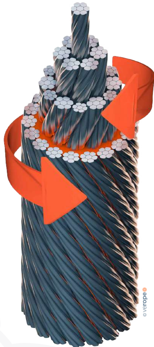
Figure 21: Rotation-resistant rope verotop P: the torques of the rope core and the layer of outer strands, generated under load, work in opposite directions.
