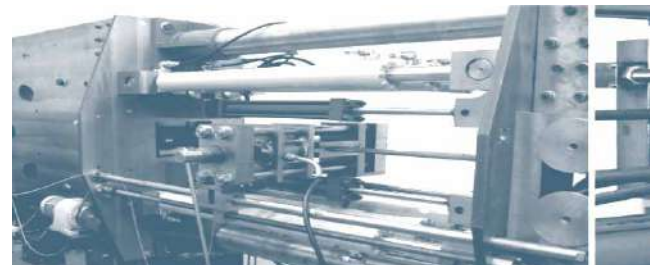
Figure 62: Testing principle of the measurement of the modulus of elasticity under load (source: TU Clausthal)
