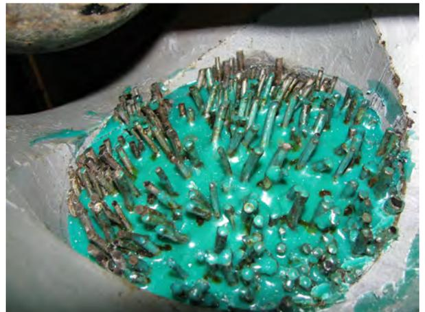
To eliminate or minimize the chance of surface cracks occurring, be careful to finish pouring the resin into the socket until it is just below the tips of the wires, and at or slightly below the top of the socket bowl. Over-topping those tips to provide a smooth even surface may look better initially, but the risk of having the assembly rejected by the customer because of their concern at the site of a crack after proof testing may be a situation you would prefer to avoid.
